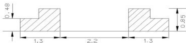
Recommended soldering pad design
